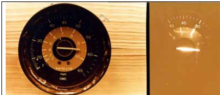
Figure 9-5 Photo of ultraviolet speedometer Source: William Chilcott
