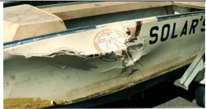
Figure 9-4 Photo of vaulted boat damage Source: Dr. William Chilcott
