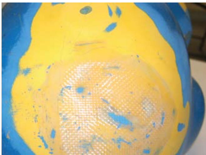
These pics show heavily damaged Kirby Morgan SL 27 hats.
